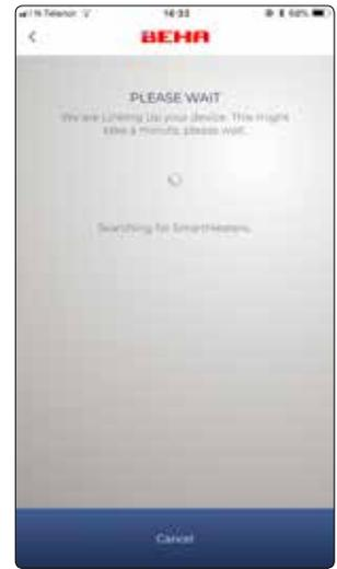
The app is now searching for the heater. Simultaneously the Wi-Fi symbol will flash on the floor. If the symbol is not flashing you have to set the heater to link-up mode. See page 7 for link-up mode.
